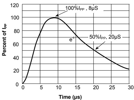
**Fig.4 Pulse Waveform-ESD(IEC61000-4-2)**
